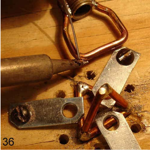
36-37. Tin one corner of the frame as shown.
