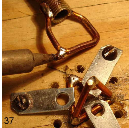
36-37. Tin one corner of the frame as shown.
